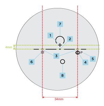
The following markings are used to verify the properties of a progressive addition lens (PAL):
